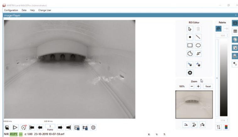
Black and white NIR-B thermal image. NIR-B offers the operator the same views as a typical CCTV system.
